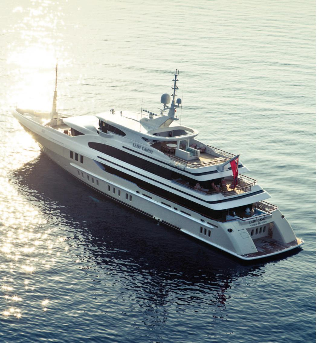
Left: Lady Candy based on a Benetti's naval platform, has been built in steel with aluminum superstructure. (photo: Jeff Brown) Length waterline at full load: 47.6 m about Overall beam: 10.60 m Total fresh water capacity: 18,000 Litres about Total fuel capacity: 130,000 Litres about Max speed, at half load condition: 15.5 knots. Cruise speed, at half load condition: 15 knots. Range at 12 knots: 5,000 nautical miles.
